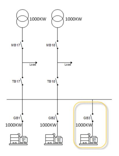
To run a power management application with short-circuit limitation, each controller in the system must have the option T1, critical power.
