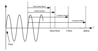
The diagram shows that when the fault has been present for two periods, the relay will trip within the specified time.
